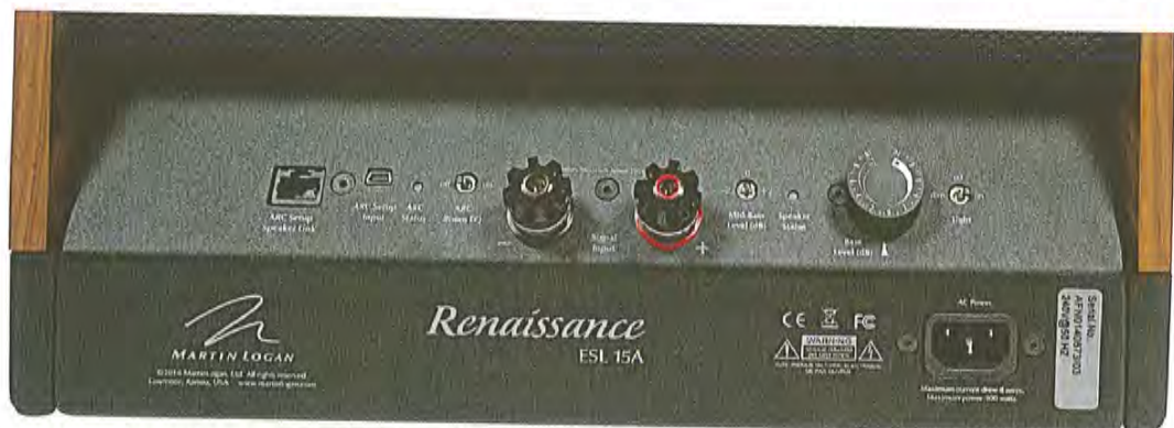
At left are an RJ45 socket for connection during room tuning, a miniUSB input for computer connection and an ARC switch. At right of the input sockets lie a small toggle switch for crossover level adjustment and at far right a light switch.
